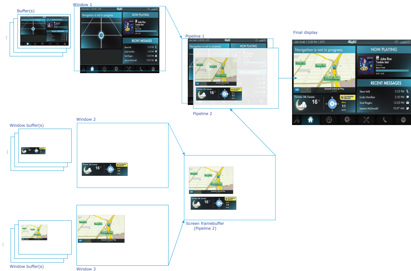
Figure 6: An example of both Screen and hardware composition with three windows, one composite buffer, and two supported pipelines
